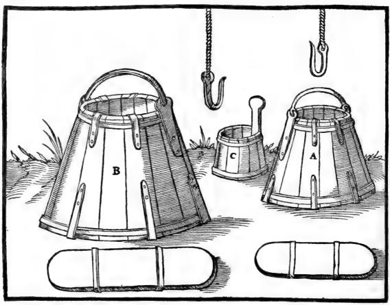
A-Smaller water-bucket. B-Larger water-bucket. C-Dipper
